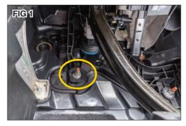
Put on safety glasses. Remove the mounting nut from firewall just to the left of the brake pedal using a 13mm socket. Save nut. (FIG 1) Next, assemble the pedal to the mounting bracket as shown. There are 3 possible different
