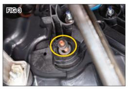
Install the supplied M8 washers over the mounting stud ad shown. (FIG 3)
