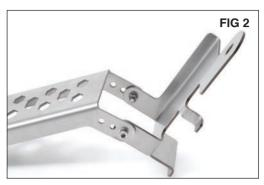
positions for height/angle options. With the M6 hardware, assemble the pedal and bracket to your desired angle/location using a 5mm hex key and 10mm open end wrench. (FIG 2)
