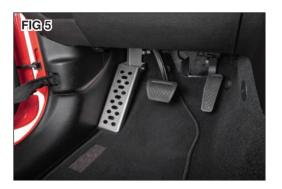
When installation is complete, be certain to verify that any floor mat or floor liner you are using does NOT interfere with your throttle or brake pedals in any way.
