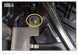
Slide the mounting bracket over the stud and re-install the original mounting nut. (FIG 4) Tighten snugly.
