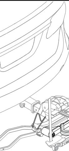
Periodically it may be necessary to adjust the tension of the swing arms. Use a 5 mm hex wrench to make the adjustment.
