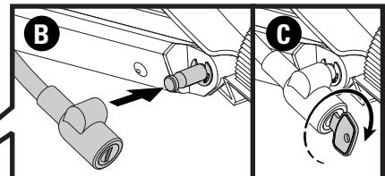
Access locking cables near the pivot arms. Pull the cable out, and pass it through one wheel, around the frame, through the other wheel, and to the lock post. Then lock it. Repeat for your other bike if applicable.
