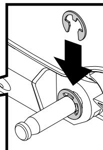
Attach the wheel cups by inserting the lock posts through the hole, front to back. Secure with e-clips.
