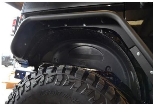
8. Do not tighten the expansion nut locations too tightly as you risk damaging the sheet metal and pulling the inserts completely out of the holes. Watch them carefully as you tighten the flares to prevent this. This completes the installation.
