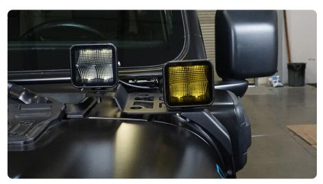
STEP 6 Using a T40 Torx bit and factory hardware, secure the DV8 A-Pillar Dual Pod Mount to the A-pillar Cowl.
