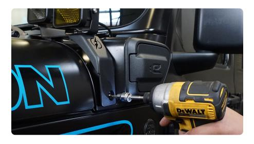
STEP 8 | Double check that all factory hardware is secure.
