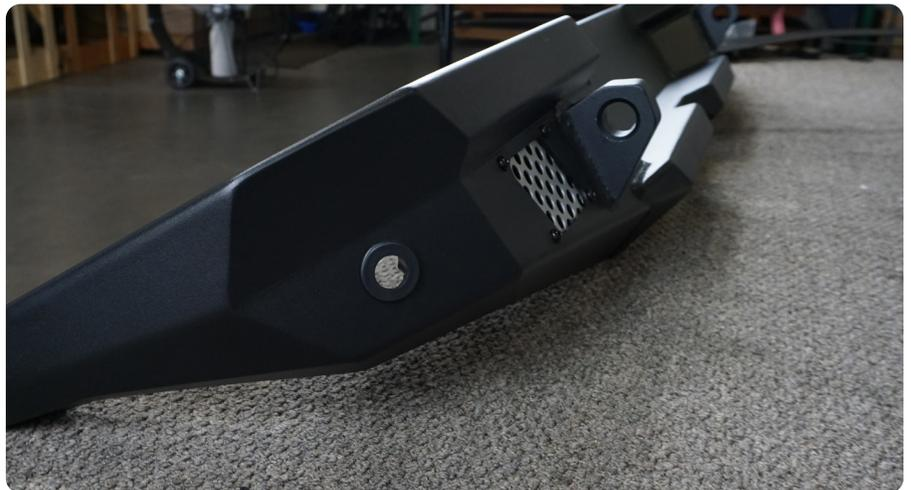
**STEP 9 |** With the bezels in place, run the sensor wiring harness through cavity in the bumper aligning the sensors with the bezels. Push Sensors into bezels ensure they have “clicked” into place. Secure sensor harness using provided zip tie tabs.
