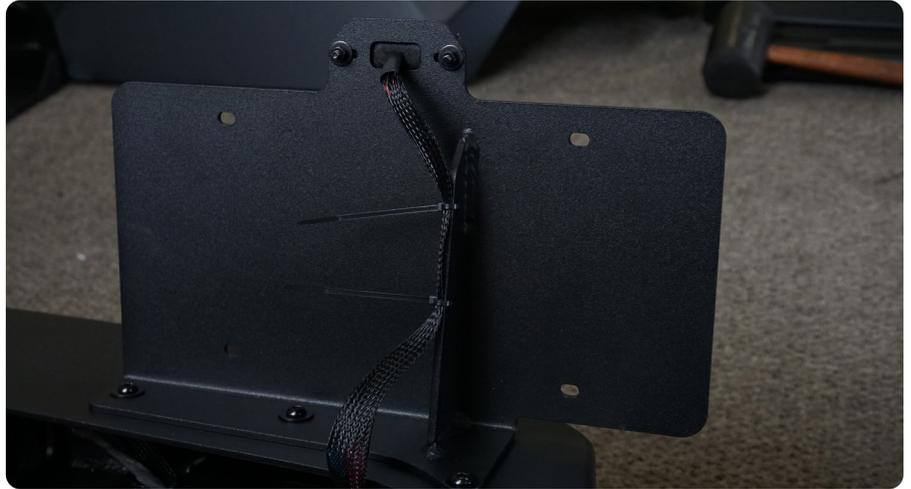
**STEP 17** | Place the provided nut plate into the passenger side of the frame with the nuts facing upwards.
