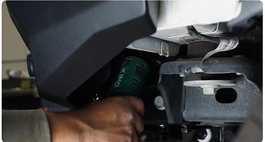
**STEP 22** | Adjust the in-and-out position of the bumper ensuring there are consistent gaps between the bumper and vehicle, and that the bumper is not touching the vehicle.
