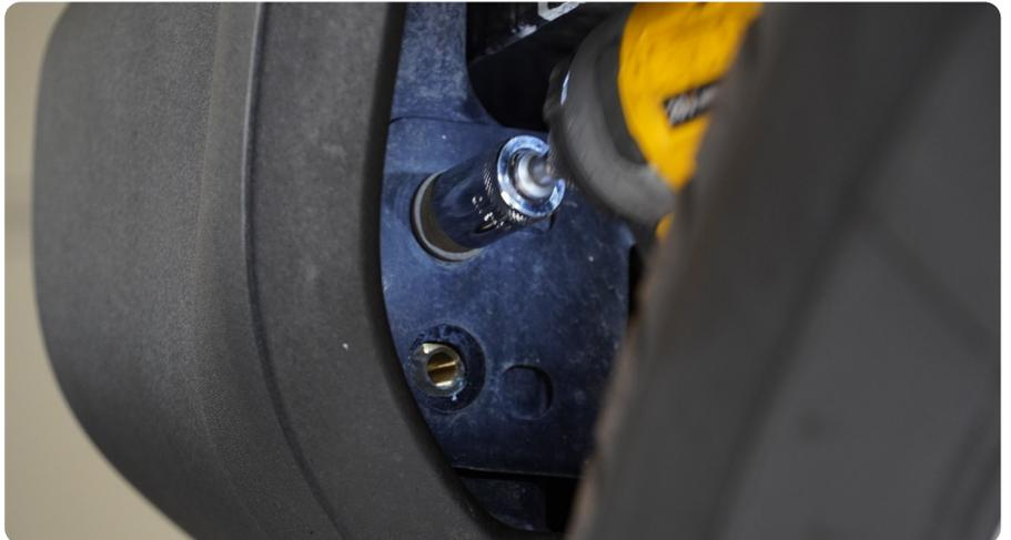
**STEP 5** | Use a 16mm socket to remove the remaining four bolts securing the bumper to the vehicle located between the bumper and rearmost body mount.
