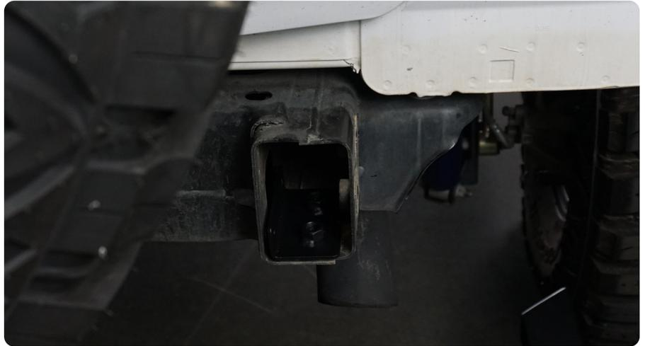
**STEP 18** | Install the clamp nuts onto the bumper.
