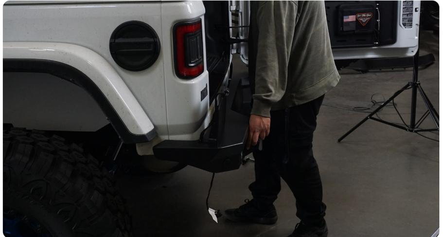
**STEP 21** | Using a 18 and 21mm socket, ensure bottom bolts are tight enough to take the weight of the bumper.
