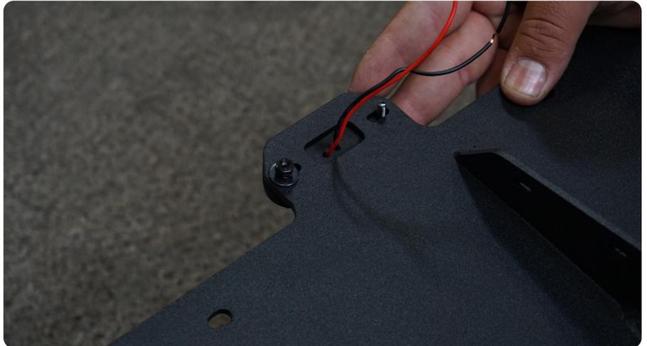
**STEP 16** | To connect the license plate light, cut off the factory license plate light plug and either cut back the factory wire loom to expose more wire length, or use 22g wire to extend the harness.
