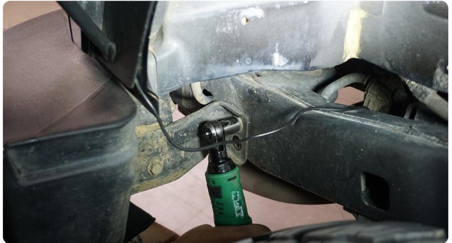
**STEP 3** | Use a 16mm socket to remove the (2) remaining bolts securing the bumper to the vehicle. Have a friend hold the bumper in place while removing this hardware.
