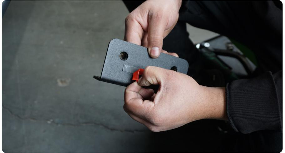
**STEP 10** | Insert and position the nut plate so it is lined up with the existing holes in the sides of the frame rail.
