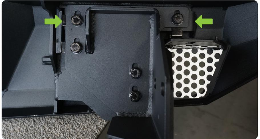
**STEP 8** | If you are installing pod lights, do so at this time using the hardware provided with the lights.
