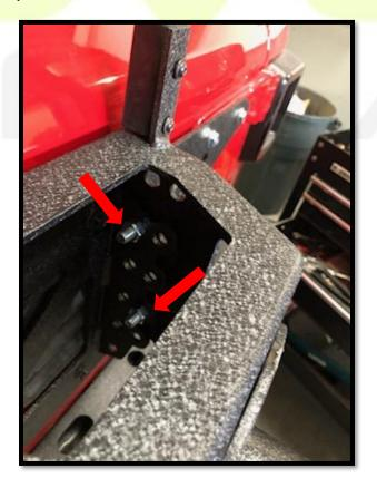
14. Tighten down (4) four tire mount bolts. Ensure all hardware is secure. Plug in camera and third bracket light. Attach tire and test door.
