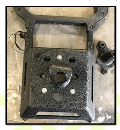
11. Place camera and camera mount inside the camera enclosure on the DV8 carrier making sure to align the 3 large holes. Utilizing the stamped stud plate from the factory tire carrier, place stud plate behind the camera mount aligning the stud through the holes.
