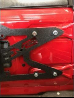
6. Once all (4) four bolts are in place, use factory hardware and remaining (8) eight spacer for bolts around tailgate exhauster vents.
