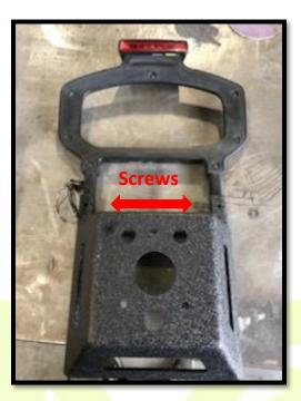
9. If you are running a rear camer<mark>a you w</mark>ill utilize the factory camera bracket (plastic) and the provided camera enclosure. If you do not have a camera, you will utilize the block off plate.
