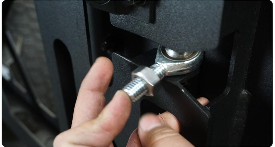
**STEP 28** | Swing the tire carrier close to the backing plate, and use the large connecting nuts to connect the backing plate to the swing arm.
