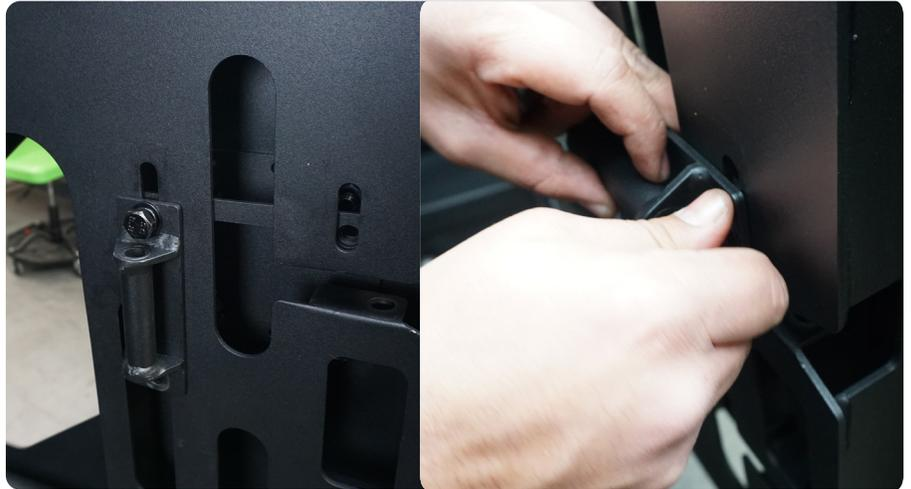
**STEP 23** | Gently close the tailgate to determine the adjustment for the tire catch.
