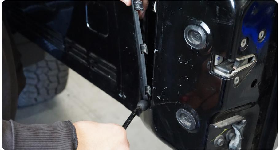
**STEP 3 |** Disconnect the third brake light wiring harness.
