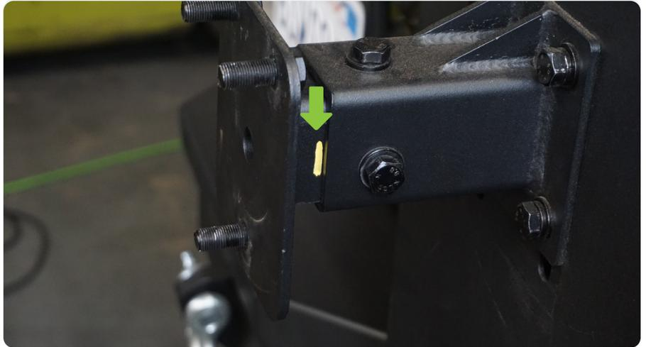
**STEP 31** | Push the carrier approximately 1/4" in from the marked line.
