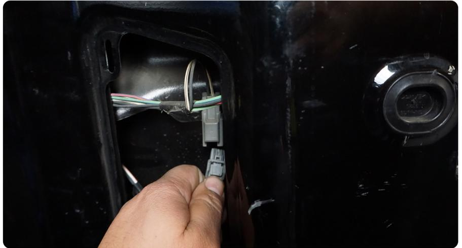
**STEP 4 |** Feed the wiring/rubber plug through to the outside of the vehicle.
