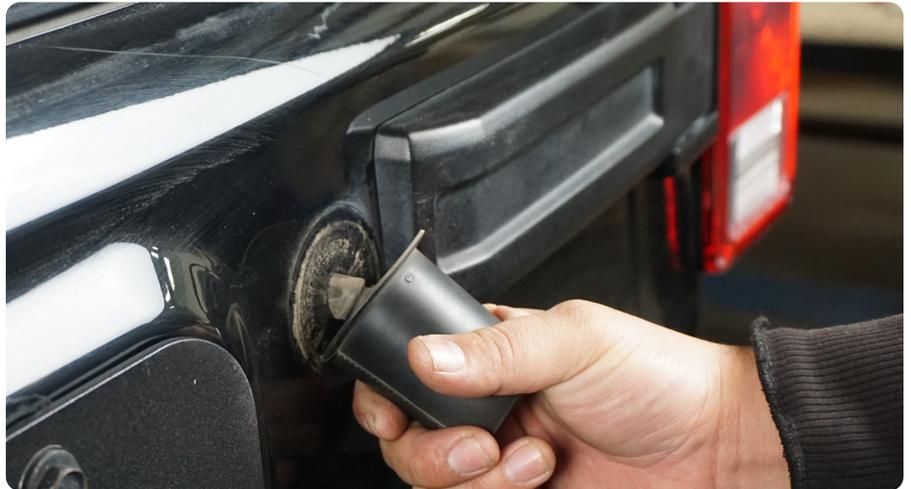
**STEP 6 |** Use a 13mm socket to remove the hardware securing the tire carrier to the vehicle, and set the carrier off to the side.
