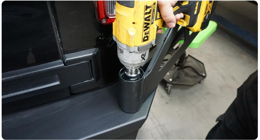
**STEP 20** | Install the M20 lock nut and flat washer on the bottom side of the spindle and secure using a 30mm socket.
