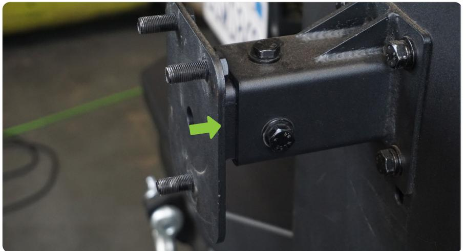
**STEP 32** | Secure the tire carrier portion of the assembly using a 16mm socket.
