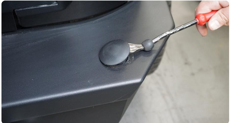
**STEP 13** | Slide the spindle through the top of the bumper.
