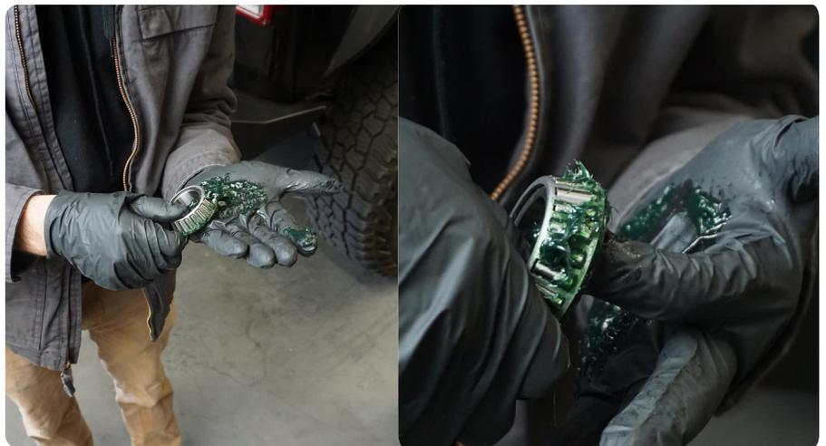
**STEP 15** | Install one of the provided bearing/race sets into the bottom of the tire carrier.
