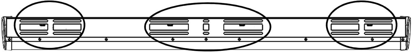
Remove the tube and install the U-nuts (N) that come with the Step Tubes into the slots identified above. Use 2 U-nuts per brace location.
