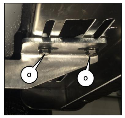
Once the tube is in the desired location, tighten hardware that connect the braces to the vehicle. Fully tighten all hardware at this time and repeat on the passenger's side.
