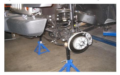
2. With the jack under the front axle, jack up the axle to remove the driver side and the passenger side wheels then disconnect the shock and sway bar end link on the driver side then the passenger side.
