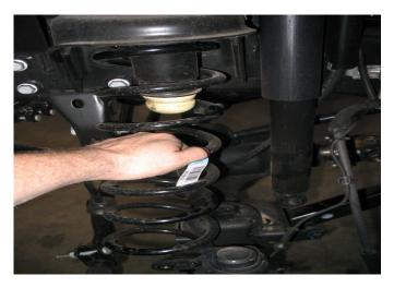
5. With the coil spring removed install new lift spacer on top of stock Spring with factory isolator pad on top of spacer.
