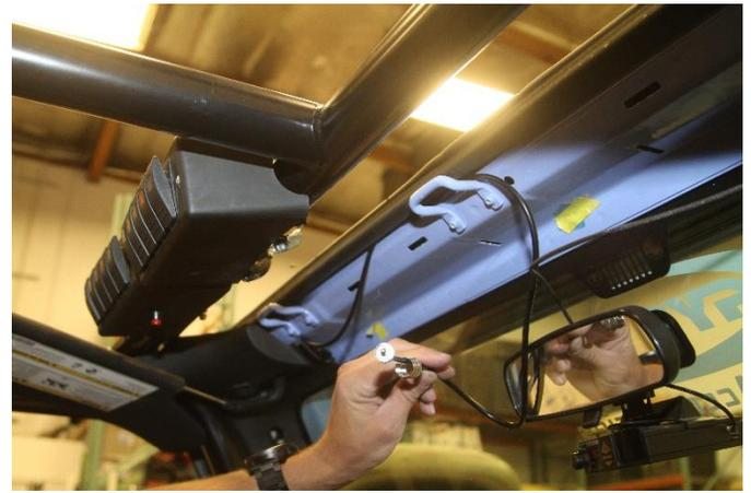
12. Install radio electrical wiring
