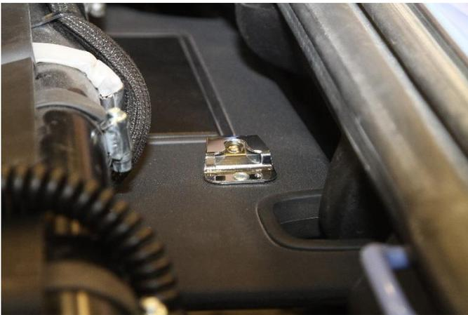
17. Firmly press mount against surface and bore out holes with a drill and bit
