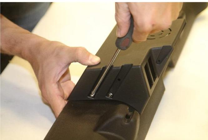
6. Install radio into corresponding hole on radio mount
