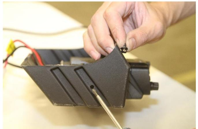
7. Install rocker switches into corresponding holes on radio mount
