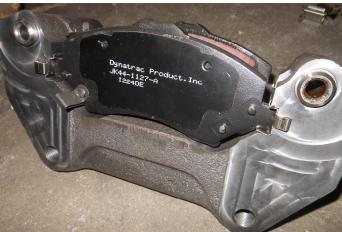
10. Fasten the Dynatrac Caliper Bracket to the Steering Knuckle with the factory bolts. Apply thread locker to the bolts and torque to 120 lb ft.
