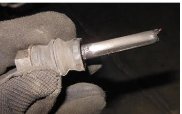
12. Once the pins are prepped and slid into the caliper bracket, the caliper can be installed onto the bracket. Take care when sliding the caliper over the new pads. Press in the caliper piston further if it will not fit over the new brake pad assembly.
