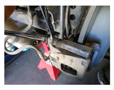
18. Next, the lower swaybar link bolt will have to be removed in order to reach the rear caliper bracket bolt.
