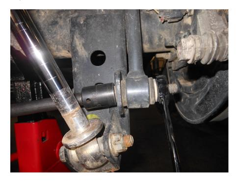
19. Now, uninstall the Stock Rear Caliper Bracket using an 18mm socket and set the hardware to the side for reuse.
