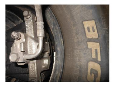
28. Once your wheels are back on the vehicle and torqued to the recommended 110 ft lbs., you should confirm that your brake fluid level is at the proper level. Test the brake pedal for pressure and make sure there are no leaks or loose bolts.
