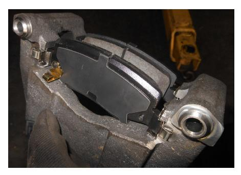
23. Once the caliper bracket is loaded, install it onto the backing plate using the factory fasteners. NOTE: Use thread locker on these bolts and torque to 77 ft lbs.
