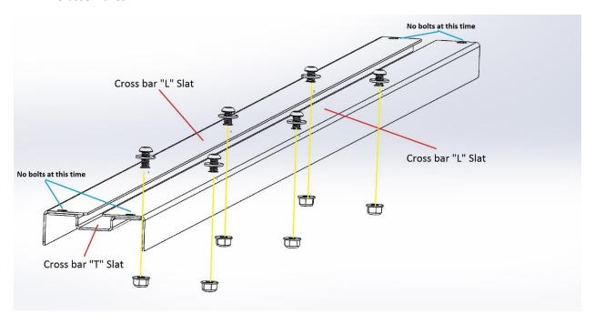
2. Assemble the front and rear slat assemblies next. These will consist of 1 "L" Slat piece and 1 "T" flat piece. Using supplied ¼" bolt, washer and flange nuts, assemble 2 sets of end (front and rear) slat assemblies by installing bolts on the 3 inner holes only. The end 2 holes and other middle 3 holes should remain without bolts at this time. Tighten 3 bolts on both front and rear assemblies. Front and rear assemblies are duplicates of each other.
