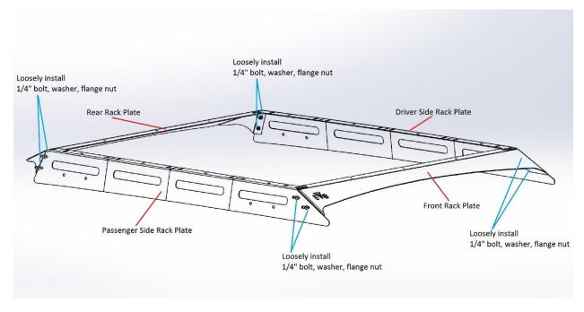
4. Using supplied ¼" bolt, washer and flange nuts, loosely install the 3 pre-assembled middle cross bar slats, front and rear cross bar slat. All cross bar assemblies should be installed on the underside of the perimeter parts.
