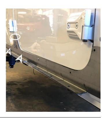
4. Follow manufacturers tool procedure and install nutserts into 4 drilled holes.
