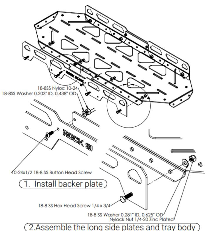
2.Assemble the long side plates and tray body
