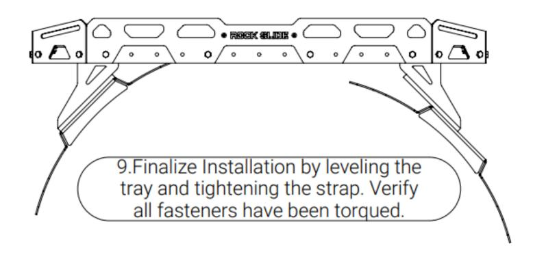
Before installing any accessories on the EZ Rack Tray, verify that your tire carrier can support the additional weight.
