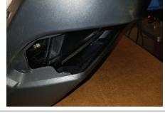
With the light removed, detach the side marker light.
