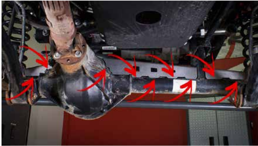
Rear weld locations
