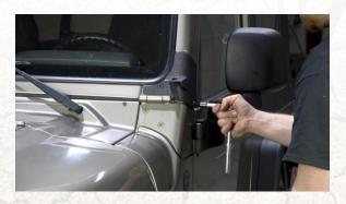
Remove the all-thread from the upper bolt location only after installing the other three (3) bolts. Install the last countersunk bolt in its place. Use the all-thread to repeat steps 1 and 2 for the opposite side.
