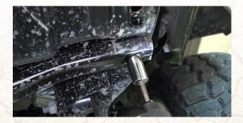
On a 2DR model, it may be required to loosen the skid plate bolt to allow enough flex to fit the new rock slider between the frame and crossbar.
