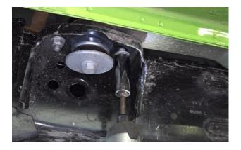
**3) INSTALL PASSENGER SIDE ROCK SLIDER** Slip the flat bracket of the rock slider between the frame and crossbar.
