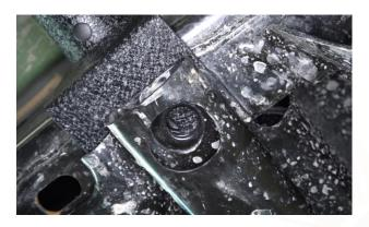
Slip the other mount(s) above the body mount washers and onto the factory studs.
