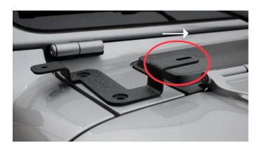
Secure it by replacing the Torx bolts and washers.
