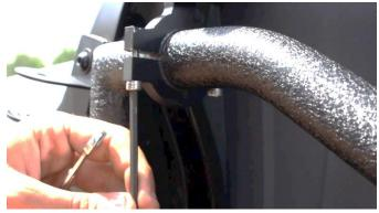
With an 8mm wrench, turn the hex nut behind the mirror clockwise so that the mirror doesn't rotate or fall.
