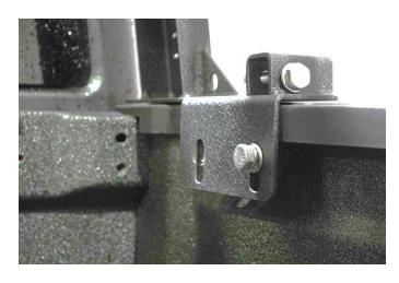
Use the included Hex bolts, lock washers, flat washers, and thread locker and secure the Bed Rack down into the T-Nuts.
