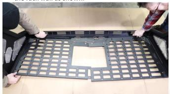
Follow the perimeter and loosely secure every bolt point with M6 bolts, washers, and flange nuts. Including the middle joined plates.
