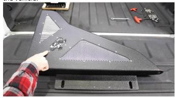
Begin applying the adhesive foam to the panel and panel brackets for both side panels.
