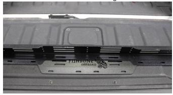
Using 4 M8 bolts, 8 flat washers, lock washer, hex nuts, and a 5mm Allen and 13mm wrench, loosely connect the cross rail to the tops of the side panels.
