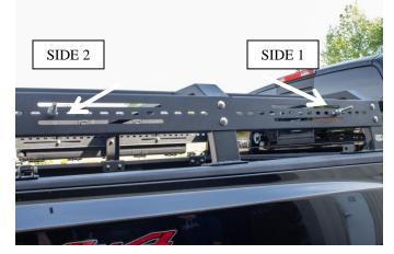
Install both threaded knobs to secure your Hi-Lift Jack to your bed rack.
