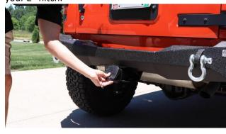
Insert the Support Bracket so that the flat side of the brackets point up.
