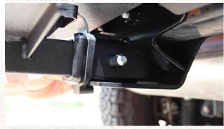
Secure the Support Bracket with the vehicle's hitch pin.
