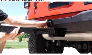
Slide it to the hitch hole which allows the closest bracket to sit about 3 inches from any above obstruction.
