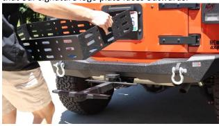
Line up the bolt holes with the Bracket's, and secure it with the included hardware and a 13mm socket and 5mm hex wrench: Bolt, washer, Basket, Bracket, washer, and Nylock nut.
