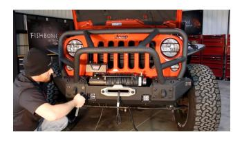
Finish the install by mounting the supplied d-rings to your bumper.
