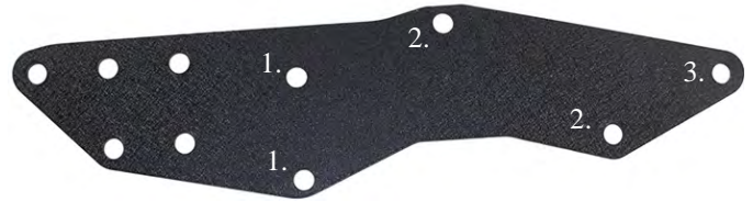
Driver side bracket – bolt location guide
