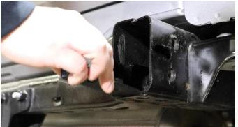
Place your rear bumper delete onto the frame, so the left and right bolt holes and slots line up.
