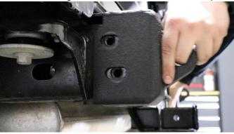
Loosely reinstall the factory bolts into their previous location, 4 21mm bolts on the driver side, and 2 18mm bolts on the passenger side. Also, loosely install the 2 provided bolts on the bottom of the frame rail on the passenger side into the nut plate.
