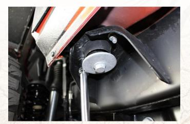
Identify the driver and passenger side. The front of the rocker guard is welded in the center of the bracket as seen below. The rears are welded offcenter of the bracket.
