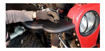
Using a ¼" bit, drill through the holes in the top of the fender to secure it to the OEM fender lip. Once again, you may want to touch up these holes with paint to prevent rust. Use the supplied hardware to secure this in place.
