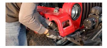
Mark a straight line up the inner back portion of your fender. This should be 1" from the outside edge of the factory fender. Again, ensuring there are no obstructions, cut along this line.
