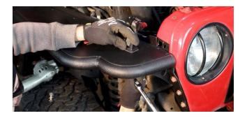
Using a ¼" bit, drill through the holes in the top of the fender to secure it to the OEM fender lip. Once again, you may want to touch up these holes with paint to prevent rust. Use the supplied hardware to secure this in place.
