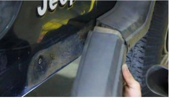
2) REMOVE FACTORY HARDWARE AND LIFT BODY Remove the three bolts holding the body to the frame. Use a 16mm socket to remove these bolts.
