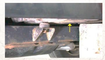
In the approximate location shown above, use a jack to lift your body away from the frame. You only need to lift a small distance to allow enough room to slide the new rock slider in place.
