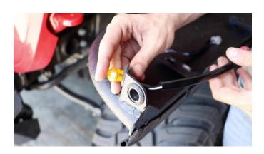
Pull the lights through and seat them into the seals so that the amber LED is furthest away from the vehicle, when right side up. Push the male connecting wires through the housing brackets/ and connect the <u>amber light to blue</u>, and the <u>white LED</u> <u>to red</u>, followed by the black and white wires to either ground connector.
