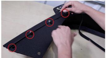
Install the included LED lights into their slots. Start by pulling the rubber seals off the lights, and firmly pushing them into the fender holes.
