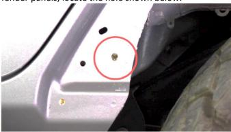
With a 7/16" drill bit, drill out the hole.
