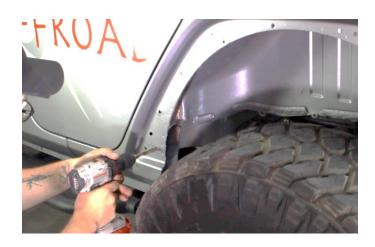
With an M8 Nutsert Tool, install a nutsert into each of the drilled holes.
