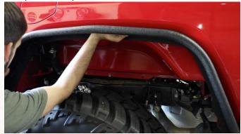
With a 5mm Allen key, tighten down the bolts.
