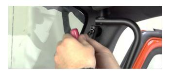
Once both bolts have been loosely installed, tighten each one a few turns at a time until they are fully tightened.
