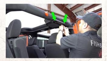
Using the supplied washer and M6 bolt, install your grab handle as shown. Tighten both bolts.
