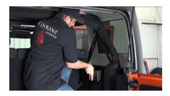
Either using all of your OEM hardware, or the supplied four (4) knobs and washers, secure the storage bins in place. Resecure your hard top.
