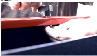
You may find it easier to hold the nut in place with a 12mm socket or wrench. You should only hand tighten the knob.
