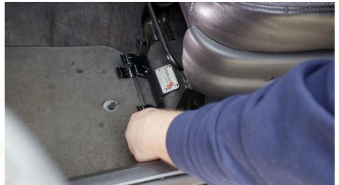
Secure it by replacing the seat bolts with a torque of 35 ft-lbs.
