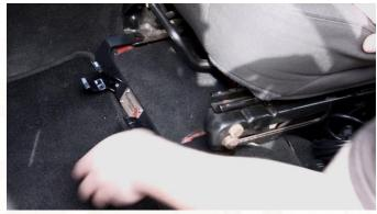
Secure it by replacing the seat bolts with a torque of 35 ft-lbs.
