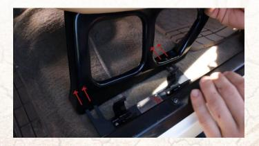
Secure it by tightening the seat bolts with a torque of 35 ft-lbs.
