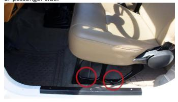
Loosen them with a 15MM Socket. Front most bolt is accessed from under the body.
