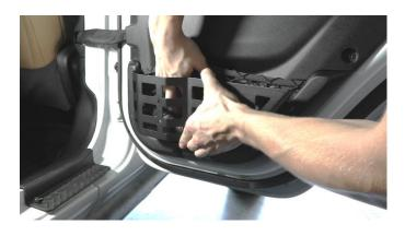
Once in place, take your hold down bracket and hook them into the slots on the bottom of your molle pocket panel. The hole on your bracket should line up with where the factory screw installs.
