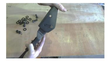
Once you have your holes aligned, screw on the included hardware. On the right side of the pedal, leave the nuts on the first few threads of the bolt. Tighten the left-side bolts to the point where the pedal does not move freely, but can be adjusted by hand. You can proceed to tighten the right-side bolts. Once again, make the bolts tight enough to where the pedal does not move freely, but can be adjusted by hand.
