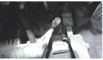
Then, adjust your pedals placement to your liking. Once you have your pedal sitting where you like it, tighten the bolts on the right side of your pedal with an 18mm socket and 19mm wrench. Due to favoring the left side of the mount in the assembly step, tightening the right-side bolts should be enough to secure the pedal.
