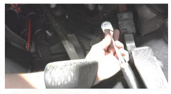
After removing the washers and nuts, take your assembled pedal and slide it onto the floorboard's bolts.
