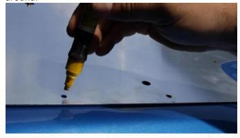
Remove the louver. With a hole punch, punch pilots into the hood to make drilling easier.
