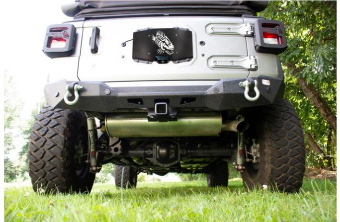
With the camera facing down place the Backside to the tailgate and secure it to the tailgate using the eight 13mm bolts.
