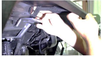
Connect the power to the vehicle and begin tightening the bolts using a 13mm wrench and 5mm Allen key. Repeat on the opposite side.
