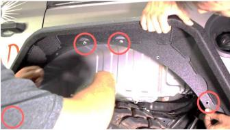
NOTE: If you choose to NOT run any inner fenders at all, you may drill out the two remaining holes shown below and secure the fender further with two more bolts, washers, and serrated nuts. We recommend against it, however.
