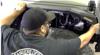
With the bolts still loose, push the turn signal power cord between the body and fender brackets.
