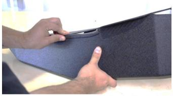
Install the included Turn Signals into each front fender. With the cord pointing towards the front of the fender, slide the signal's tab behind the front bracket while rotating it down and into the rear bracket. Secure the signals to the fender using a 3mm Allen wrench with the included M5 bolts, washers, and serrated nuts.
