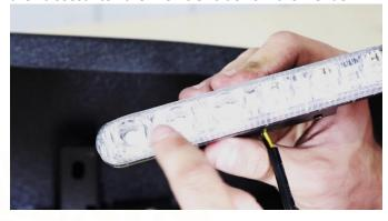
Push it into the bracket, pulling the wire through it, and secure it to the bracket with the 2 longer m5 bolts, washers, and nuts.
