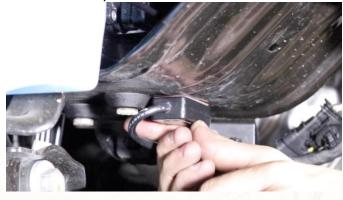
With the fender installed, test the alignment of the light. Move the light around as desired and secure its angle by tightening the vertical and horizontal bolts with a 3mm allen.
