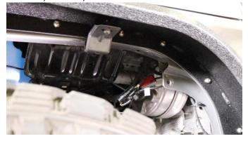
Connect the turn signal's power to the vehicle. Remove the tape backing on the power converter and secure it to your vehicle as desired.
