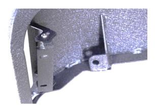
Next, insert the light through the slot and into the bracket so that the LEDs with the directional lenses are closest to the vehicle side of the fender.
