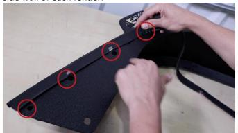
Install the included LED lights into their slots. Place the retaining bracket in between the fender brackets, and loosely secure it with 2 of the smaller m5 bolts, washers, and nuts.
