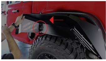
Slide your front inner fenders into the well and align the holes behind the body and into the nutsert.
