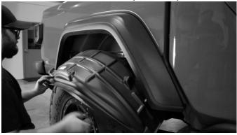
Inside the wheel well, at the shown hole, with an M8 Nutsert tool, install one of the included nutserts into the vehicle.
