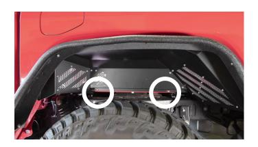
With a 3mm allen and two of the included M6 bolts, washers, and serrated nuts, secure the bottom of the fender.
