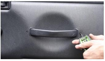
To remove the handle, simple pull it out and away.
