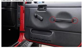
With a T15 Torx bit, remove these two bolts and washers.
